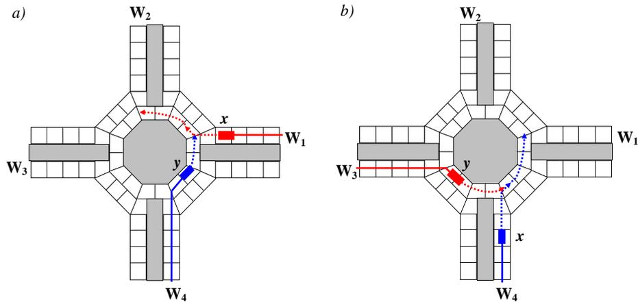
Fig. 2. The collision situation in case the vessel on the roundabout is a) on the lateral lane (has no priority) b) on the main lane (has priority)
