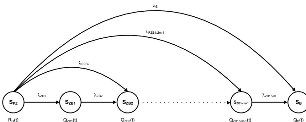
Fig. 4. Relationships within highway emergency response system in case of two or more alarm indicator column failure, where:  $\lambda_{RZB}$  – transition rate of two or more alarm indicator columns
