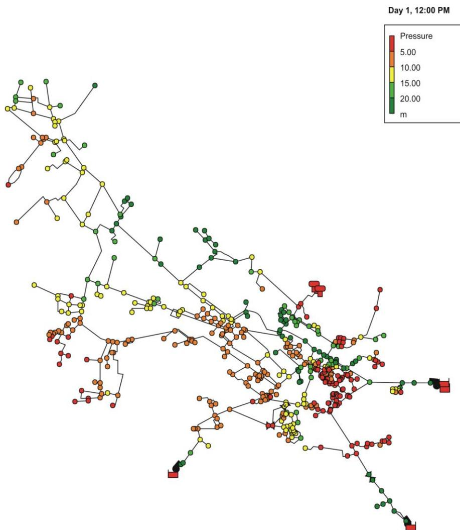
Fig. 3. Simulation of 5th hour of pipeline ND 500 failure
