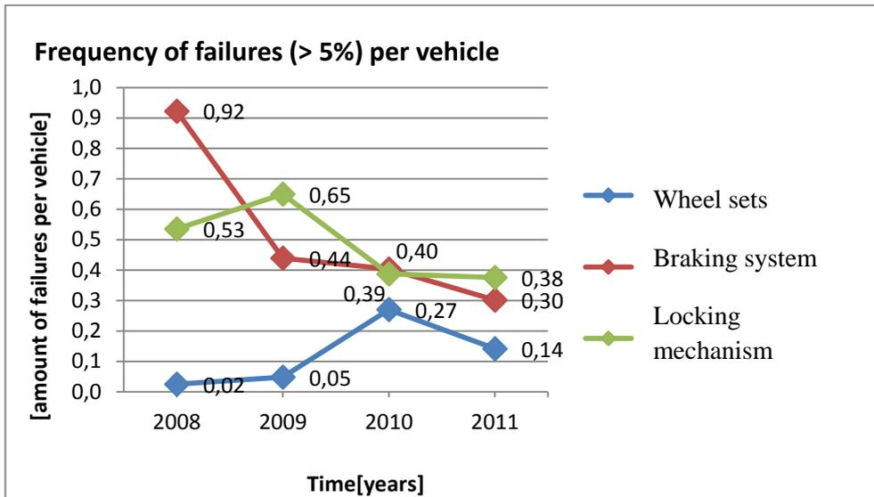
Fig.4. Amount of failure types per wagon in years
