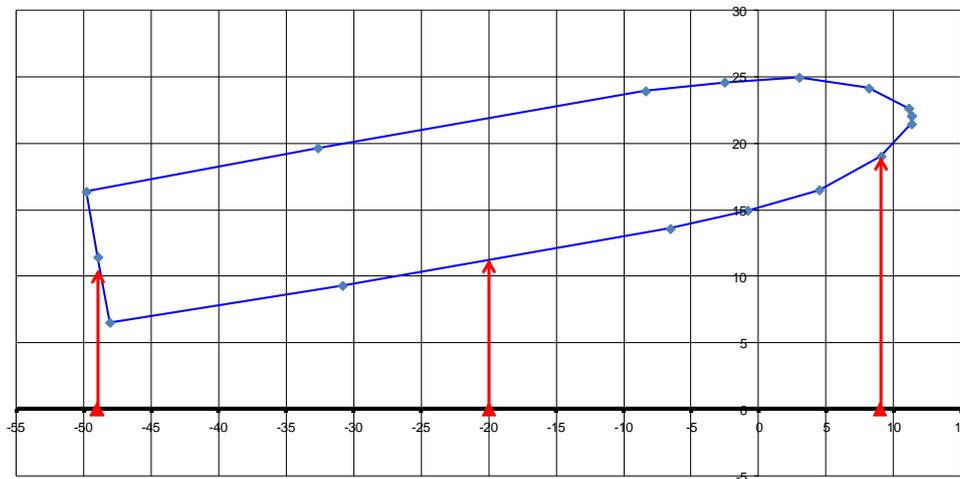
Fig. 3 Principle of measurement from three laser range sensors in PNDS
