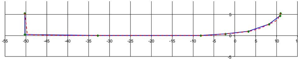
Fig. 2 The spline approximation of m/s "Nawigator XXI" half plane contour
