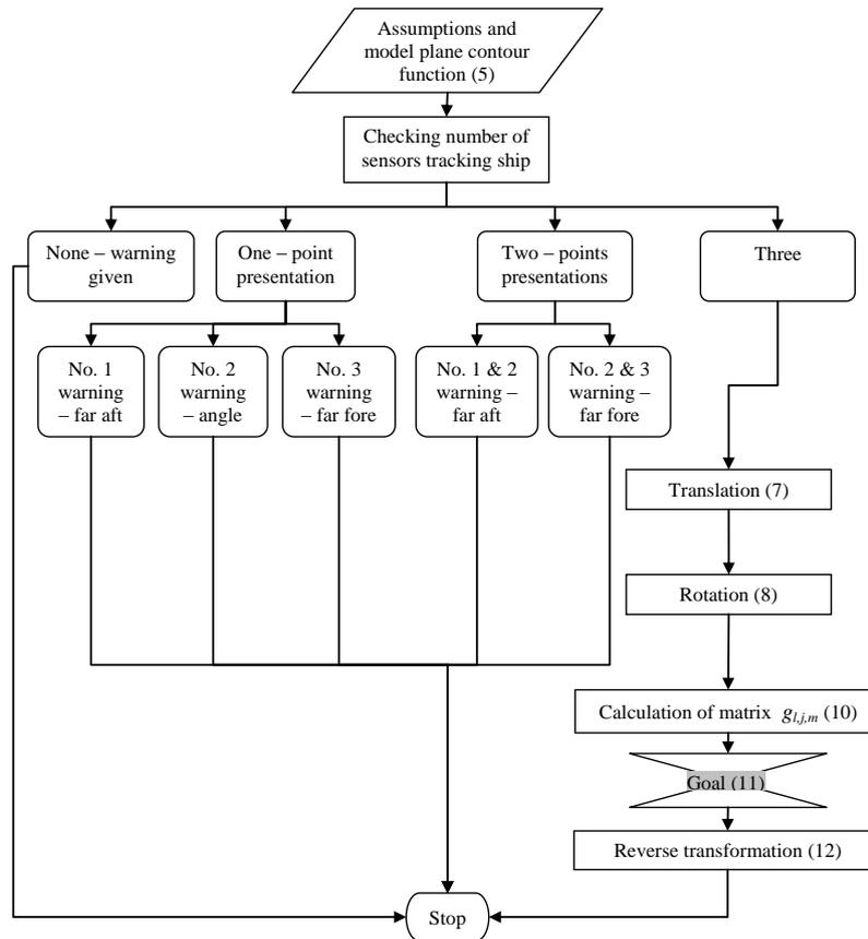
*Fig. 4 Algorithm of ship's horizontal plane determination from three laser range sensors in PNDS*
