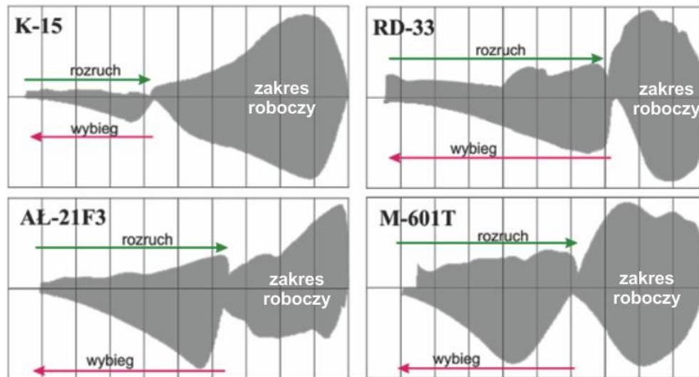
*Fig. 4. Phase portraits for rotational speeds of engines*
